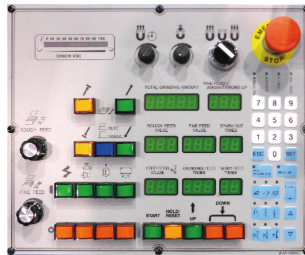
AUTOMATIC DOWNFEED AD5 (NC) CONTROL PANEL (optional)
