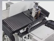
• Instead of using hydraulic driving system, the regulating wheel is driven by linear motor. This improves dressing speed and stable control.
