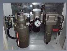
• Oil mist lubrication device aids wheel spindle lubrication, clean and constant
