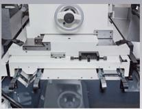
● The one "V" & one flat feeding slide design reinforces the feeding stability. The entire feeding slide is hand scrapped to reduce friction and to increase accuracy of jog movement.
