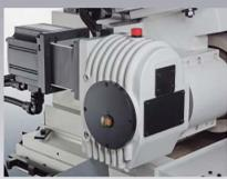
• Adjustable worm shaft eliminates the gap, increases transmission efficiency and lifetime.
