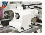
The rigid tailstock is locked on the slide firmly. The tailstock quill movement is driven by hydraulic power for convenient and fast workpiece clamping and unclamping.
