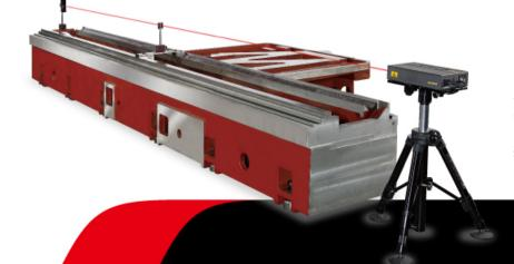
The slide way adopts scraping technics processing, inherits traditional techniques, cooperates with precise measuring equipment, and ensures the smoothness and straightness on the slide way with rigorous demand.
