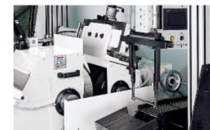
11. Auto. loading and unloading attachment (infeed grinding)
